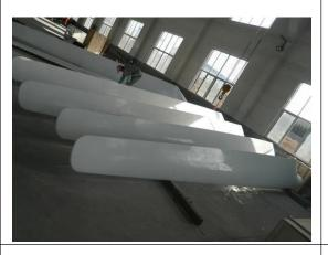
**Material of blades:** High efficiency FRP material, ultraviolet prevention rosin, plus unidirectional high strength glass fiber, modernization craft vacuum cast technique synthesis.
